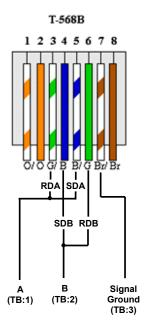
Figure 30: PU Port Connections
